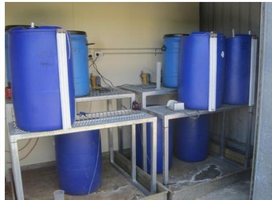
*Figure 1 (left) – Bottle roll testwork on Barnes Hill saprolite samples
